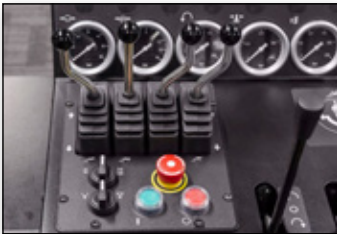
Complete drill and boom controls
